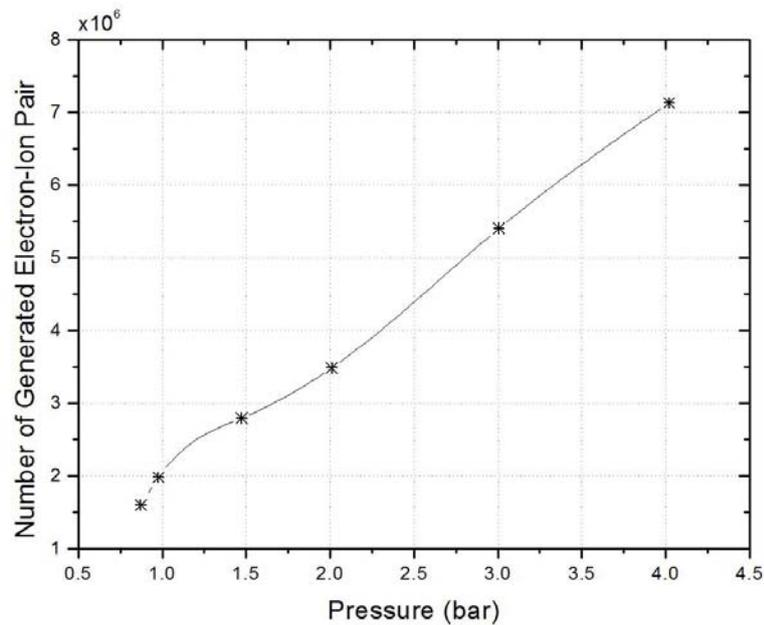
Fig. 1. The variation of electron-ion pair production vs. pressure
