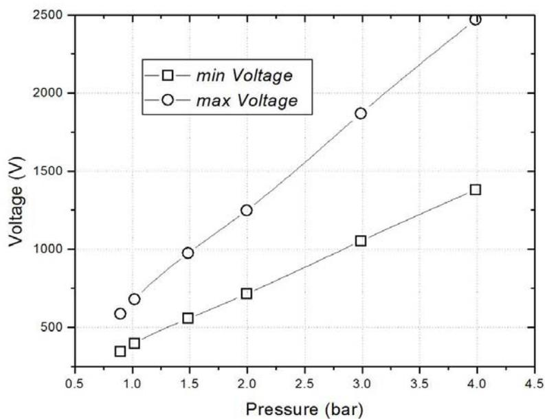
Fig. 2. The variation of Vmin- Vmax plateau voltage vs. internal gas pressure
