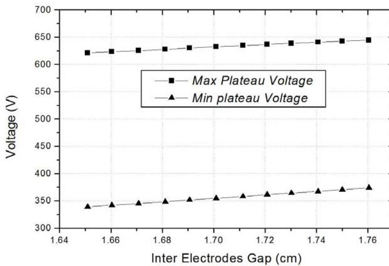
Fig. 6. The variation of min and max plateau voltages vs. inter-electrodes gap
