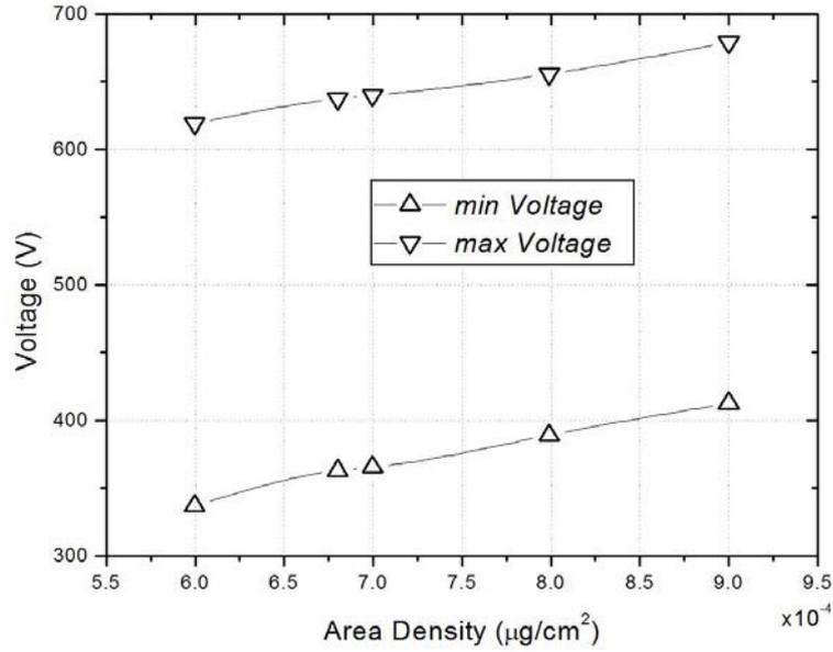
Fig. 3. The variation of Vmin-Vmax plateau voltage vs. surface mass
