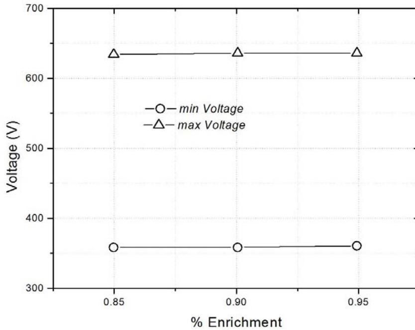
Fig. 5. The variation of min-max plateau voltage vs. enrichment
