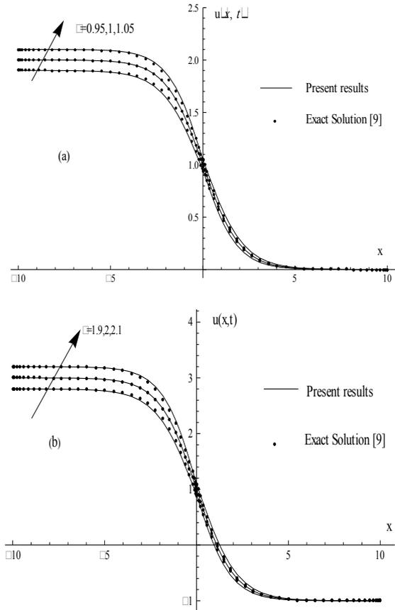
**Fig. 2.** Comparison with Burgers equation at different values of  $\nu$  and  $a_1 = 0.001, a_1 = -1$
