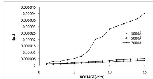
**Fig. 7.** Variation of Photo-current with voltage for  $\text{Cu}_2\text{S}$  film of different thickness for constant illumination
