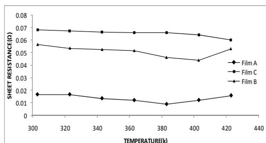
**Fig. 12.** Variation of sheet resistance with temperature for  $\text{Cu}_2\text{S}$  film of 7000 Å thickness at different annealing temperature
