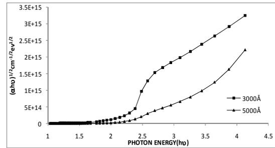
**Fig. 5.** Variation of absorption coefficient with photon energy for Cu<sub>2</sub>S films of different thickness
