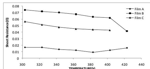
**Fig. 10.** Variation of sheet resistance with temperature for  $\text{Cu}_2\text{S}$  films of 3000Å thickness at different annealing temperature
