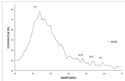
**Fig. 1.** X-ray diffraction spectra of  $\text{Cu}_2\text{S}$  films of 3000 Å thickness
