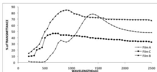
**Fig. 9.** Variation of transmittance spectra with wavelength for  $\text{Cu}_2\text{S}$  films of 3000 Å thickness at different annealing temperature
