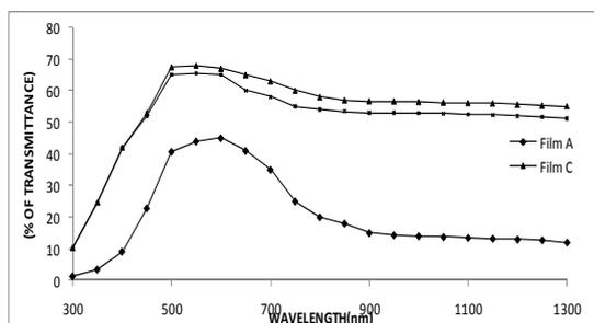
**Fig. 11.** Variation of transmittance spectra with wavelength for  $\text{Cu}_2\text{S}$  films of 7000 Å thickness at different annealing temperature
