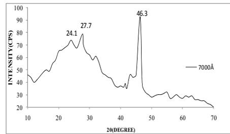
**Fig. 3.** X-ray diffraction spectra of  $\text{Cu}_2\text{S}$  films of 7000 Å thickness
