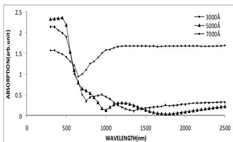
**Fig. 4.** Absorption spectra of Cu<sub>2</sub>S films of different thicknesses
