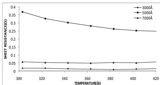
**Fig. 6.** Variation of sheet resistance with temperature for  $\text{Cu}_2\text{S}$  film of different thickness
