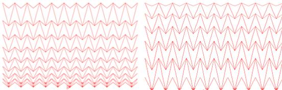
**Fig. 2.** Double arrowhead FGM structure
