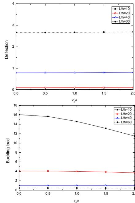
Fig. 6. Effects of nonlocal parameter on the deflection and buckling load of isotropic beam
