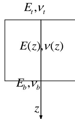
**Fig. 5.** Variation of material properties through the thickness direction of FGM beam
