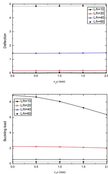
**Fig. 8.** Effects of nonlocal parameter on the deflection and buckling load of FGPR beam
