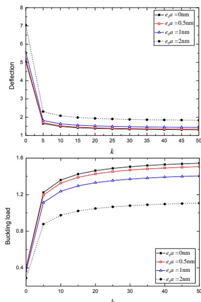
**Fig. 9.** Effects of gradient index on the deflection and buckling load of FGPR beam
