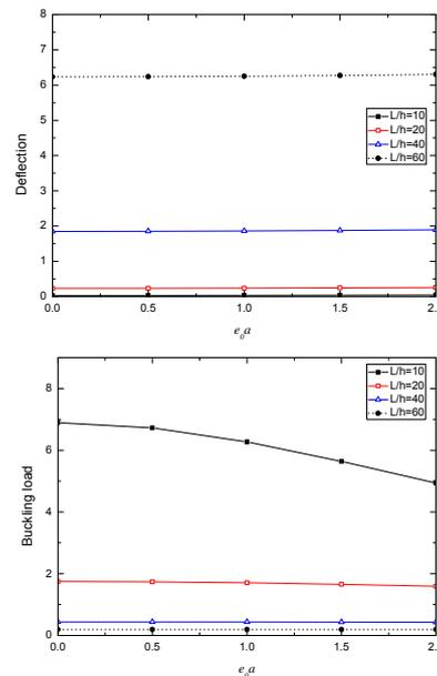
Fig. 7. Effects of nonlocal parameter on the deflection and buckling load of FG beam with constant Poisson's ratio
