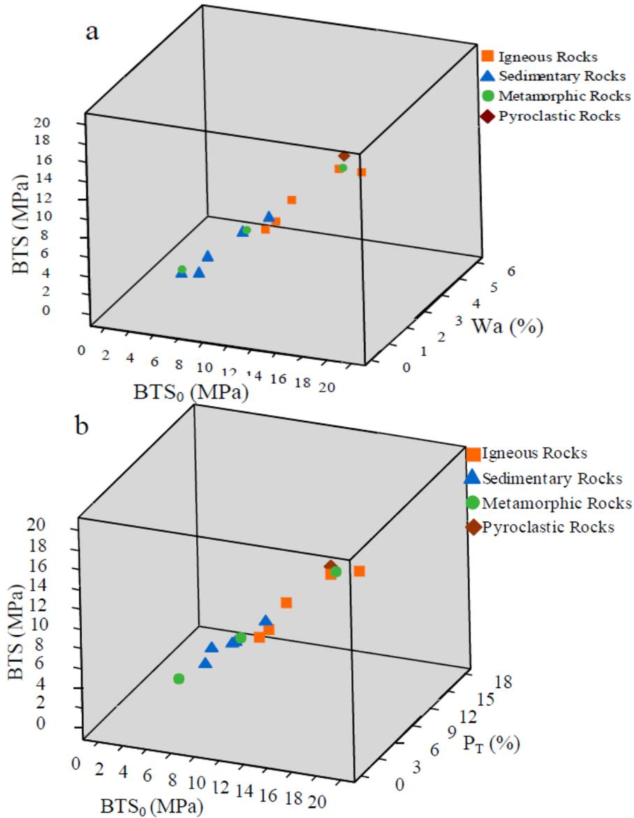
**Fig. 5.** The regression models after (a)  $BTS = -1.215 - 0.343 W_a + 1.008 BTS_0$  and (b)  $BTS = -0.595 - 0.125 P_T + 0.973 BTS_0$  with scattered experimental data
