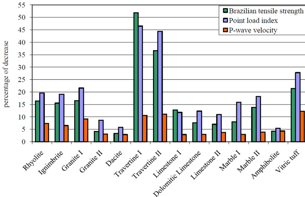
Fig. 1. The percentage of decrease in the samples' engineering properties after freeze-thaw action
