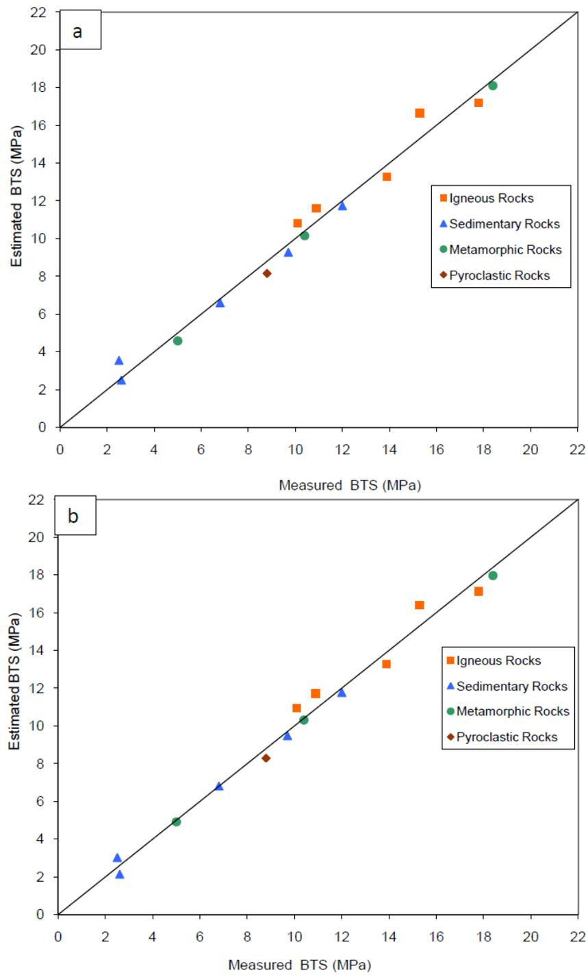
**Fig. 8.** Measured BTS versus estimated BTS from (a)  $BTS = -1.215 - 0.343 W_a + 1.008 BTS_0$  (b)  $BTS = -0.595 - 0.125 P_T + 0.973 BTS_0$
