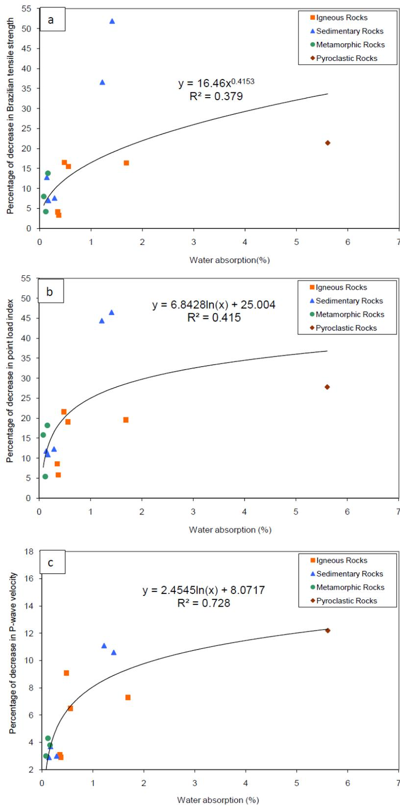
**Fig. 2.** The relationship between the samples' water absorption and the percentage of decrease in their (a) Brazilian tensile strength (b) point load index (c) P-wave velocity after freeze-thaw action
