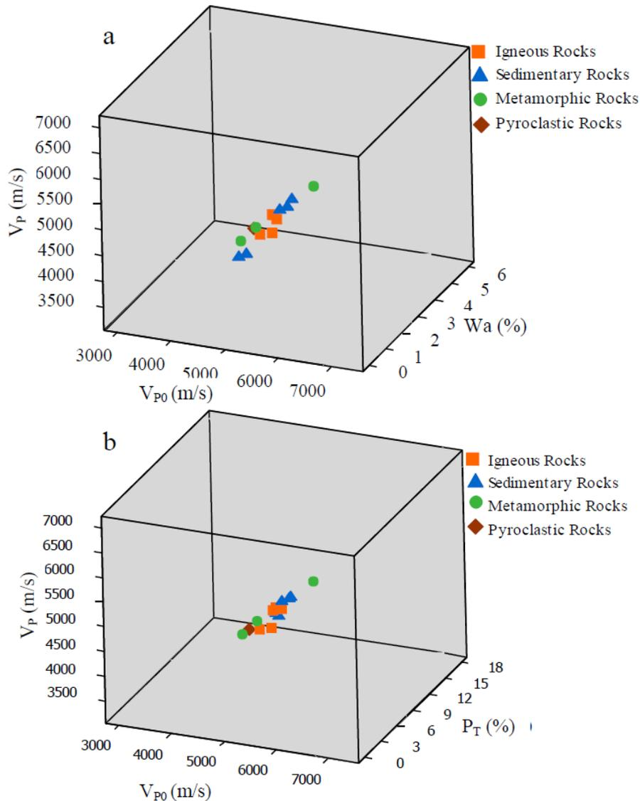
**Fig. 7.** The regression models after (a)  $V_p = -832.194 - 13.382 W_a + 1.097 V_{p0}$  and (b)  $V_p = 55.027 + 27.28 P_T + 0.954 V_{p0}$  with scattered experimental data
