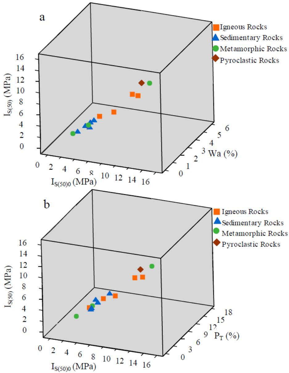
**Fig. 6.** The regression models after (a)  $I_{s(50)} = -0.759 - 0.277 W_a + 0.983 I_{s(50)0}$  and (b)  $I_{s(50)} = -0.430 - 0.095 P_T + 0.957 I_{s(50)0}$  with scattered experimental data
