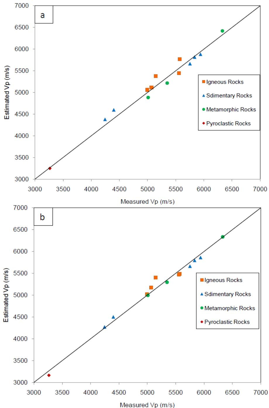
**Fig. 10.** Measured  $V_p$  versus estimated  $P_w$  from (a)  $V_p = -832.194 - 13.382 W_a + 1.097 V_{p0}$  and (b)  $V_p = 55.027 + 27.28 P_T + 0.954 V_{p0}$
