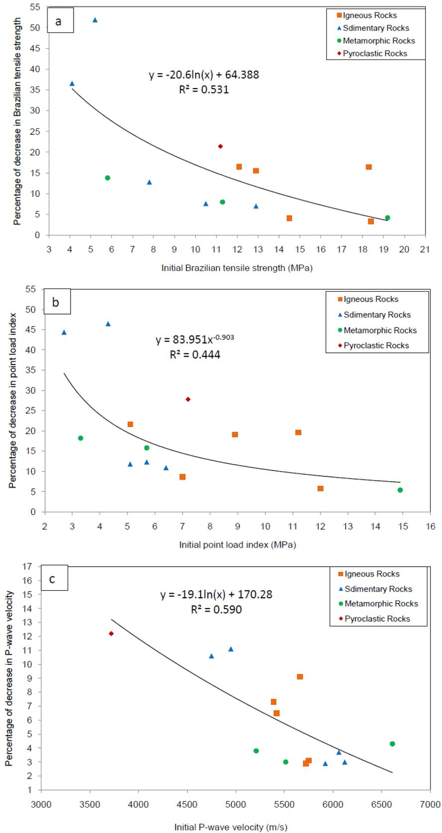
**Fig. 4.** The relationship between the percentage of decrease in the samples' (a) Brazilian tensile strength and their initial values (b) point load index and their initial values (c) P-wave velocity and their initial values
