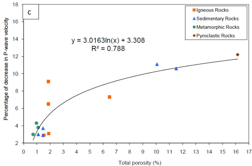
**Fig. 3.** The relationship between the samples' total porosity and the percentage of decrease in their (a) Brazilian tensile strength (b) point load index (c) P-wave velocity after freeze-thaw action
