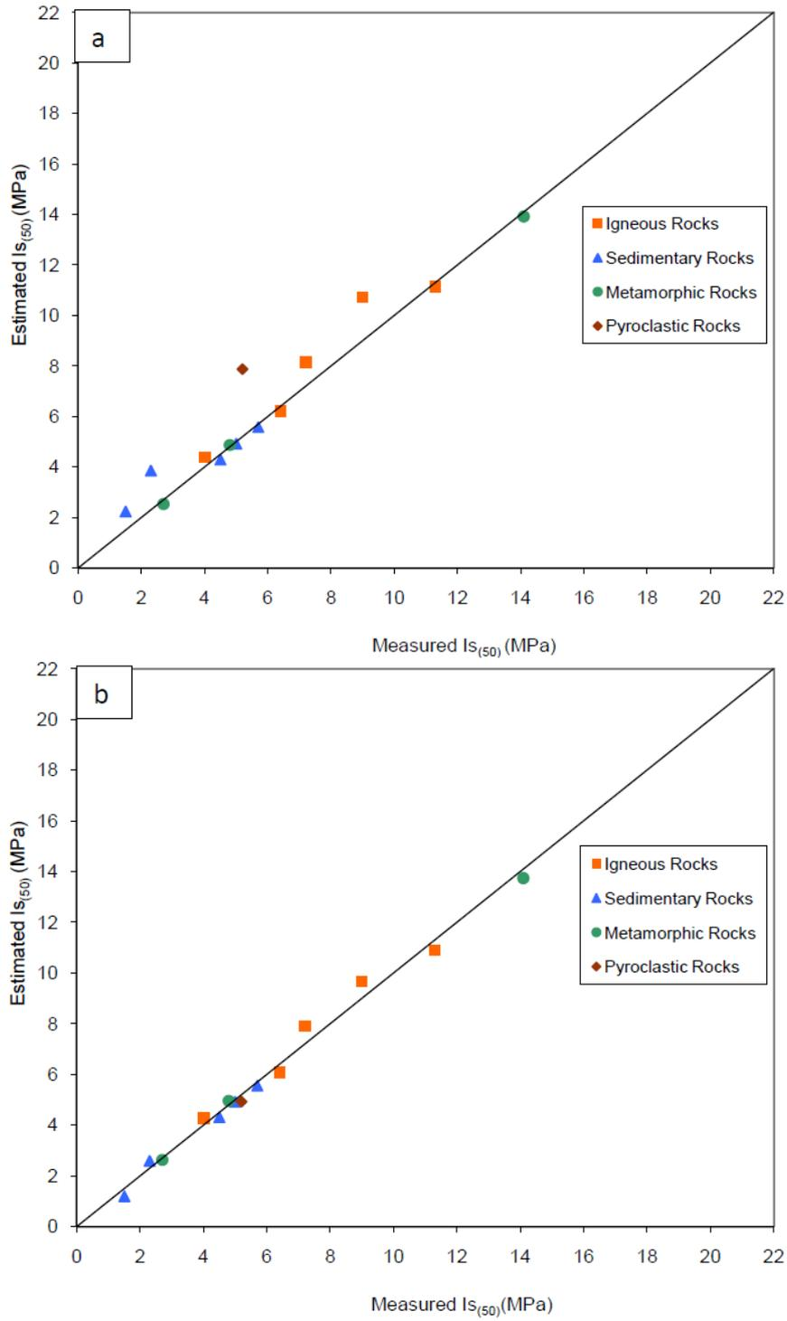
**Fig. 9.** Measured  $I_{s(50)}$  versus estimated  $I_s$  from (a)  $I_{s(50)} = -0.759 - 0.277 W_a + 0.983 I_{s(50)}$  and (b)  $I_{s(50)} = -0.430 - 0.095 P_T + 0.957 I_{s(50)}$
