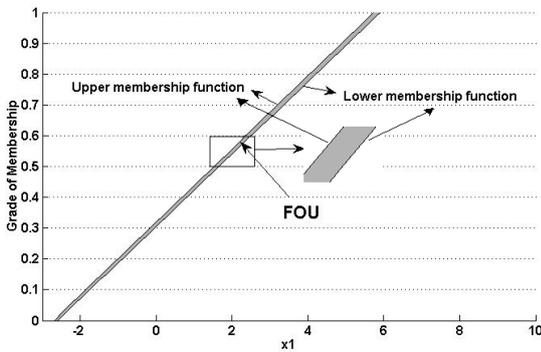
**Fig. 3.** Plot of  $\mu_{\tilde{M}_1^2}(Z_1(x(t)))$ , Lower membership function  $\underline{\mu}_{\tilde{M}_1^2}(Z_1(x(t)))$ , Upper membership function  $\overline{\mu}_{\tilde{M}_1^2}(Z_1(x(t)))$  and footprint of uncertainty (grey area) for Genesio-Tesi system
