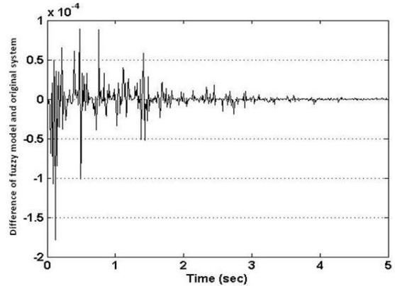
**Fig. 4.** Modeling error for Genesio-Tesi system
