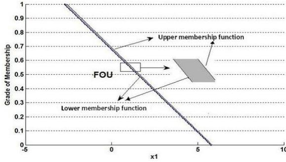
**Fig. 2.** Plot of  $\mu_{\tilde{M}_1^1}(Z_1(x(t)))$ , Lower membership function  $\underline{\mu}_{\tilde{M}_1^1}(Z_1(x(t)))$ , Upper membership function  $\overline{\mu}_{\tilde{M}_1^1}(Z_1(x(t)))$  and footprint of uncertainty (grey area) for Genesio-Tesi system
