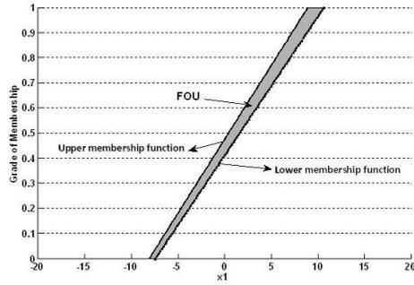
**Fig. 7.** Plot of  $\mu_{\tilde{M}_1^2}(Z_1(\mathbf{x}(t)))$ , Lower membership function  $\underline{\mu}_{\tilde{M}_1^2}(Z_1(\mathbf{x}(t)))$  (dashed line), Upper membership function  $\bar{\mu}_{\tilde{M}_1^2}(Z_1(\mathbf{x}(t)))$  (filled line) and footprint of uncertainty (grey area) for Rossler system
