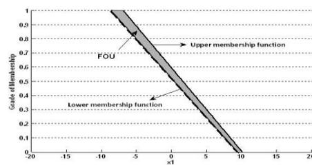
Fig. 6. Plot of  $\underline{\mu}_{M_1^1}(Z_1(\mathbf{x}(t)))$ , Lower membership function  $\underline{\mu}_{M_1^1}(Z_1(\mathbf{x}(t)))$  (dashed line), Upper membership function  $\bar{\mu}_{M_1^1}(Z_1(\mathbf{x}(t)))$  (filled line) and footprint of uncertainty (grey area) for Rossler system
