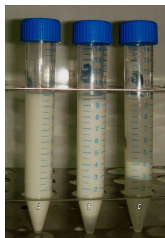
Fig 4. Breaking of water/Kerosene emulsion by whole culture of Ochrobacterum anthropi strain RIP15-1 following assay incubation time (h). A, model water/Kerosene emulsion; B, the mixture consisting of model water/Kerosene emulsion and medium C; C, reaction mixture consisting of model water/Kerosene emulsion and cell-free culture filtrate of strain RIP15-1
