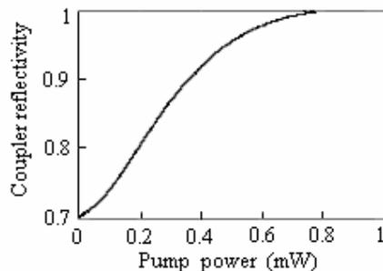
Fig. 4. Curve of the coupler reflectivity  $r$  as a function of the pump power  $P$
