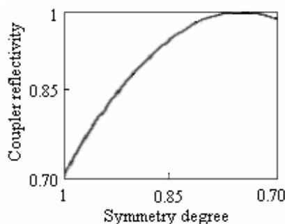
Fig. 3. Curve of coupler reflectivity  $r$  as a function of symmetry degree  $\psi$  for  $\kappa L = 3\pi/4$
