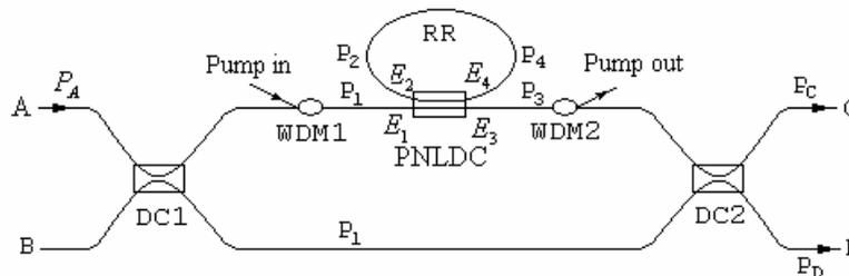
Fig.1. M-Z interferometer optical switch with a ring resonator coupled by a PNLDC
