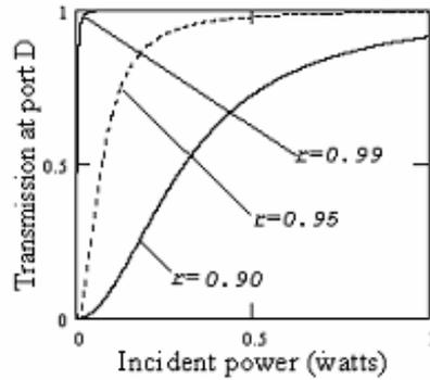
Fig. 2. Curve of output transmission at port  $D$  as a function of incident power for different  $r$
