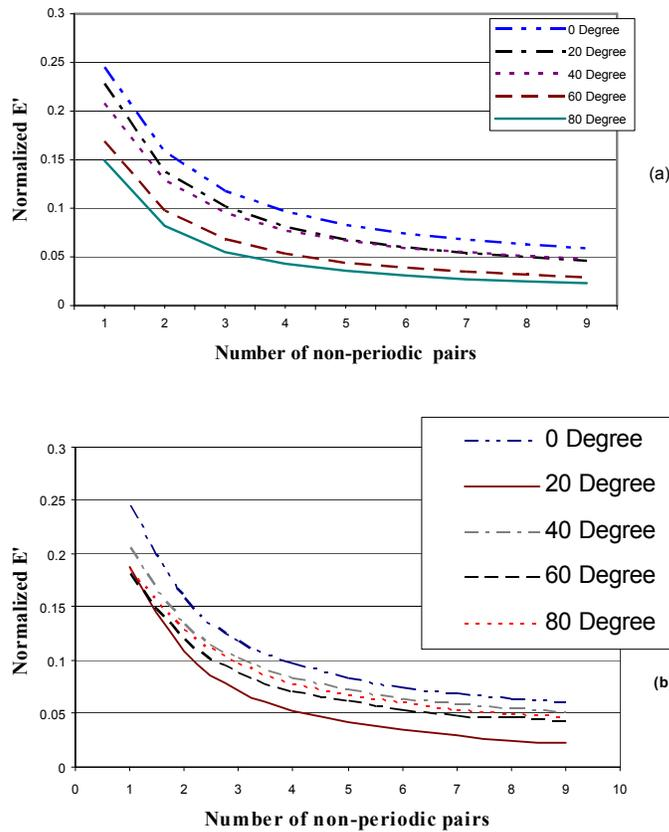
Fig. 5. The peak of the electric field  $E'$  for normal and oblique incidence versus the number of non-periodic pairs, using the “substrate scheme” design for: (a) polarization S, and (b) polarization P
