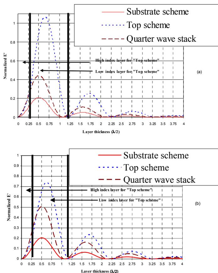
Fig. 3. The electric field within the optical layers for a laser beam with an incident angle of  $40^\circ$  with: (a) polarization S, and (b) polarization P
