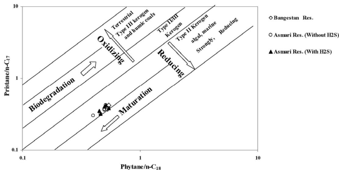
Fig. 5. Pristane/n-C<sub>17</sub> versus Phytane/n-C<sub>18</sub> showing the marine source (type II Kerogen with strongly reducing environment) for Asmari and Bangestan Reservoir oils in Marun Oilfield (After Connan & Cassou [24])
