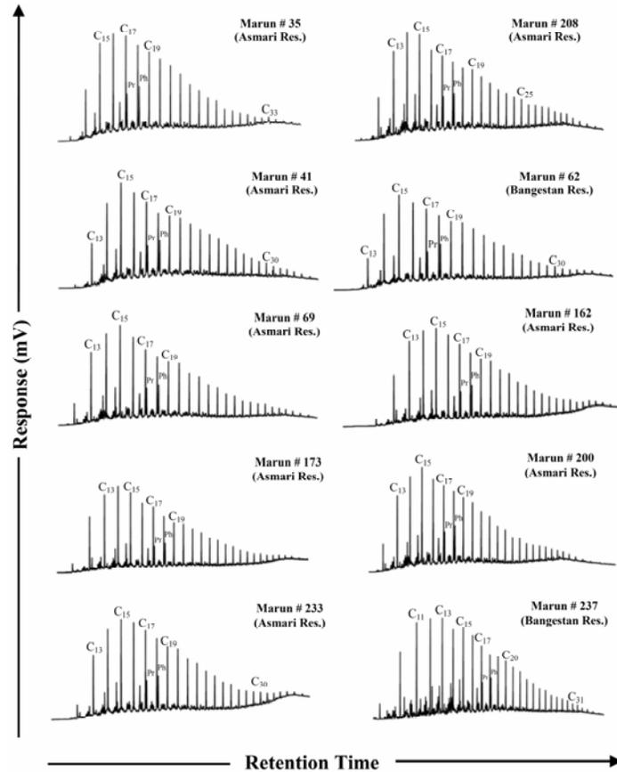
Fig. 4. Gas Chromatography of the whole oil of 10 oil samples in the Marun oilfield
