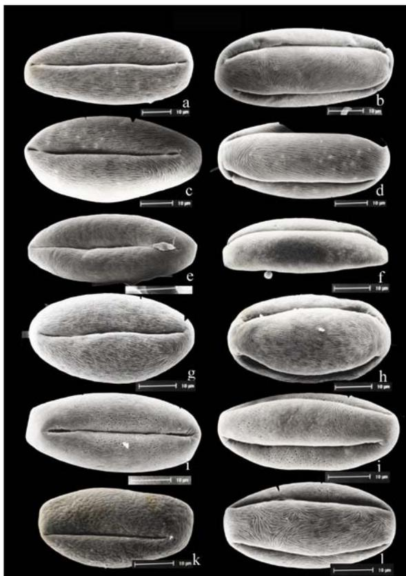
Fig. 3. Scanning electron micrograph of pollens of *Malus* species. a, b: *M. coronaria* (a, side view; b, equatorial view); c, d: *M. glaucescens* (c, side view; d, equatorial view); e, f: *M. ioensis* (e, side view; f, equatorial view); g, h: *M. platycarpa* (g, side view; h, equatorial view); i, j: *M. trilobata* (i, side view; j, equatorial view); k: *M. lancifolia* (side view); l: *M. tschonokii* (equatorial view)
