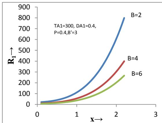
**Fig. 5.** Variation of Rayleigh number  $R_1$  with dimensionless wave number  $x$  for different values of suspended particles parameter  $B$
